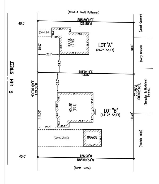
SCALE: 1"=30' LEGEND O = SET 5/8" CAPPED REBAR • = FOUND IRON PIPE M = MEASURED DISTANCE
