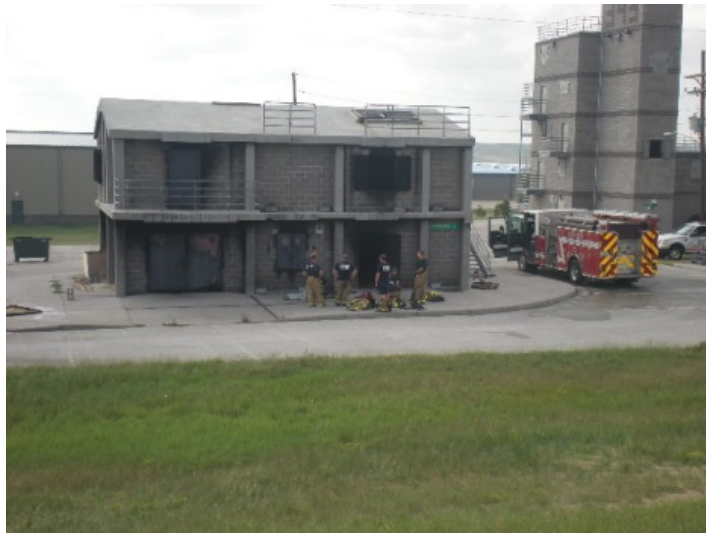
Example of a burn structure with two levels. A deck on the back serves as an entry-point for “basement” fire. A ventilation prop may be seen on each pitch of the roof.
