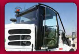
Heavy-duty guards surround cab and protect sweeper by guiding lowhanging tree limbs up and over the Pelican. Available in right hand, left hand, or dual configuration.
