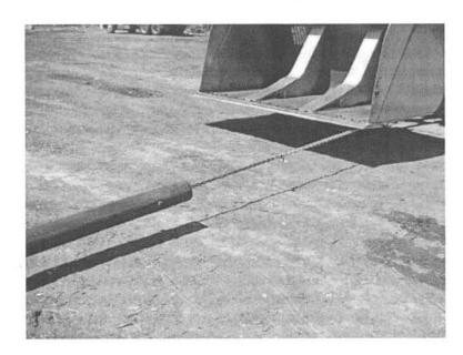
The air lances are removed using a front end loader before the pile is moved. This allows the piping to be reused and allows rapid movement of the pile itself.
