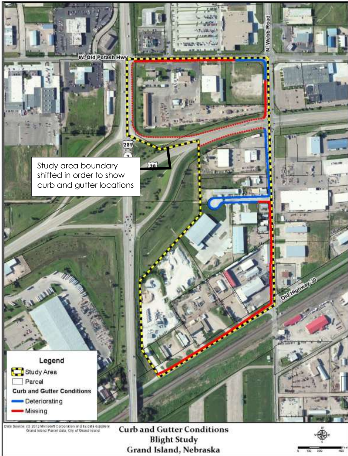
Figure 5 Curb and Gutter Conditions
