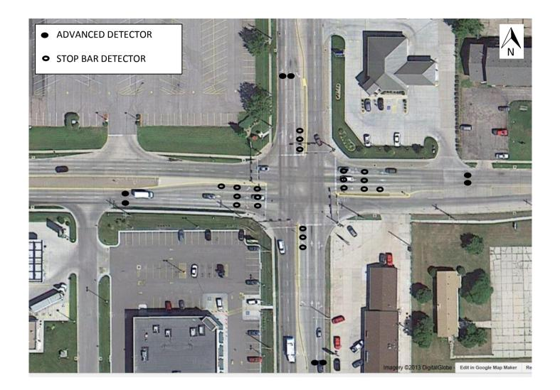
\*LOCATIONS ARE APPROXIMATE. LAYOUT ABOVE IS FOR GENERAL GUIDANCE ON INTERSECTION GEOMETRICS AND QUANTITY/TYPE OF DETECTORS.
