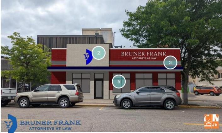
PROPOSED FINISH MATERIALS AS INDICATED: 1. ENDICOTT FACE BRICK, 2. BURNISHED CONCRETE BLOCK, 3. PAINTED STEEL CHANNEL REVEAL, 4. PRECAST CONCRETE VENEER, 5. INSULATED GLAZING, 6. MAPES PREFINISHED METAL CANOPY W/ TIE-RODS
