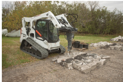
Example of Skid Steer/Compact Track Loader
