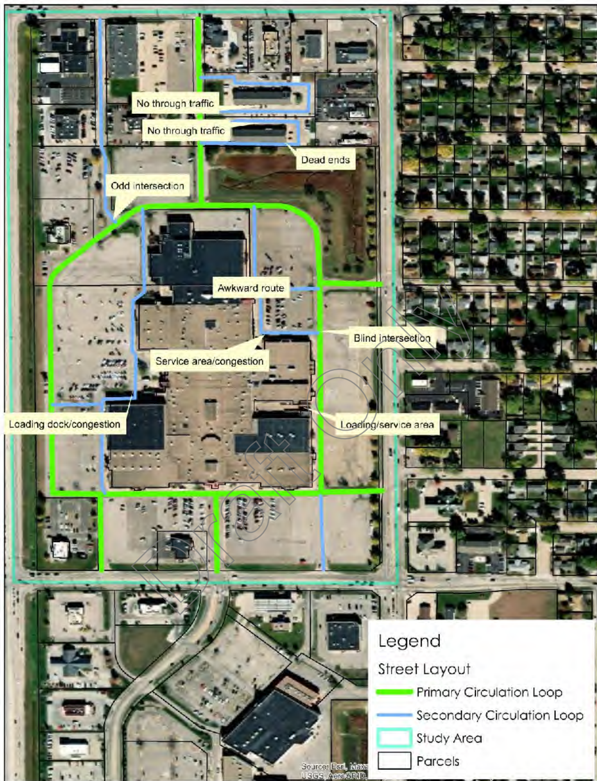
Figure 8 Defective Street Layout
