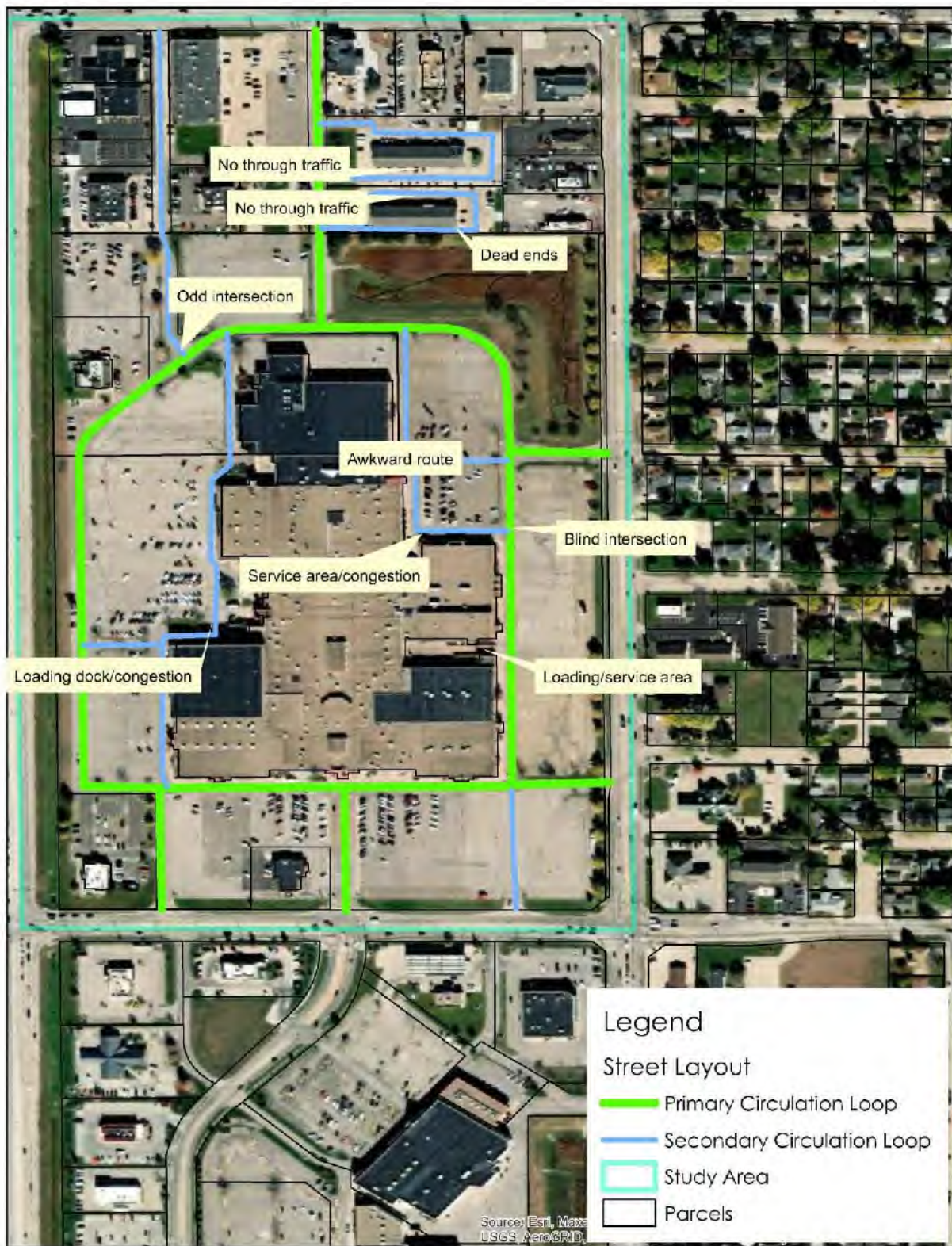
Figure 8 Defective Street Layout
