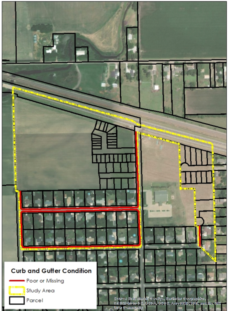
Blight Study - Curb and Gutter Condition Grand Island, Nebraska
