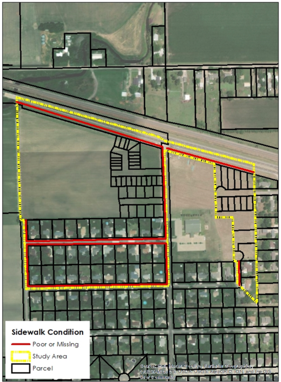
Blight Study - Sidewalk Condition Grand Island, Nebraska
