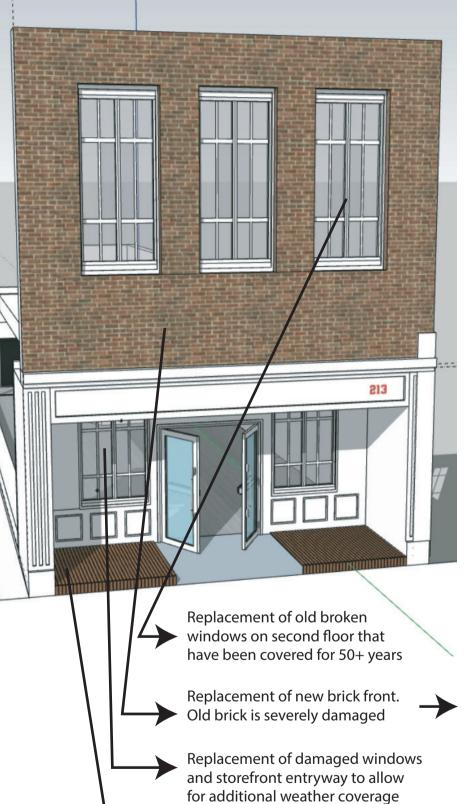
Restructure landing of entryway to fix broken concrete and allow for recessed window space.
