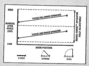
The Magic-Force" delivers consistent opening force. Fully field adjustable to meet specific site conditions. Easy opening with a powerful close. Patent pending.
