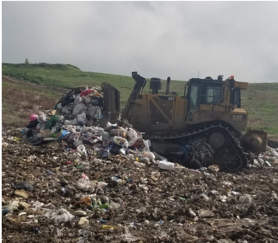
Picture of the D8T Dozer at work in the Landfill
