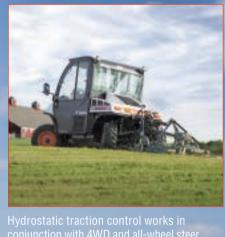
Hydrostatic traction control works in conjunction with 4WD and all-wheel steer, minimizing turf damage or loss of traction in soft ground conditions.
