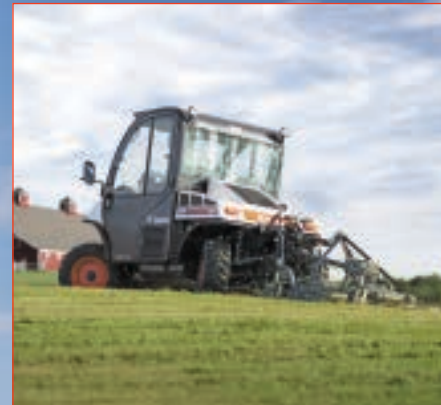
Hydrostatic traction control works in conjunction with 4WD and all-wheel steer, minimizing turf damage or loss of traction in soft ground conditions.
