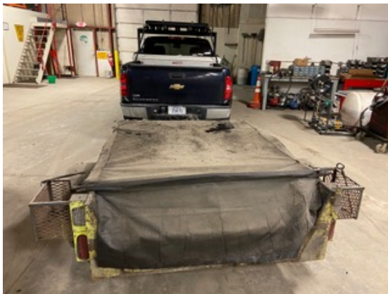
Existing cold patch trailer setup with hose connected to exhaust for heat source.
