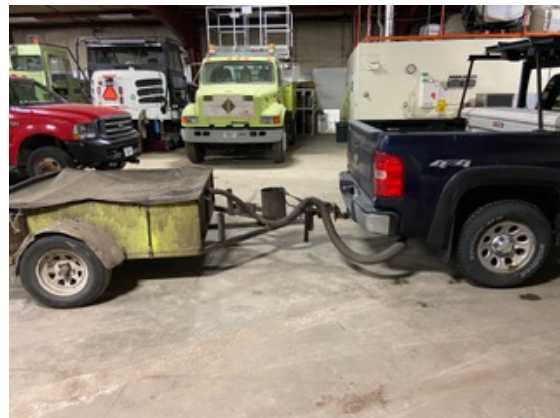
Existing cold patch trailer setup with hose connected to exhaust for heat source.
