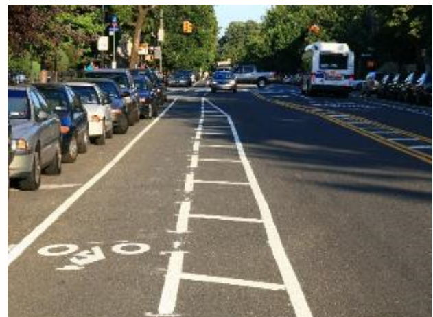
Figure 4-27 Buffered Bike Lane
