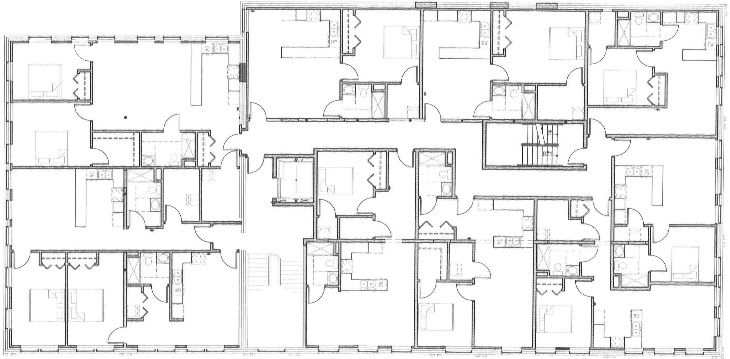
SECOND FLOOR PLAN 3/16" = 1'-0" 0 2'-0" 4'-0" 8'-0" SCALE: 3/16" = 1'-0"
