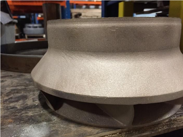
4. Impeller wear turn.
