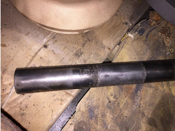
1. Worn and pitted journal turns on pump shaft.
