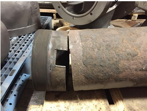
8. Cut column for disassembly.
