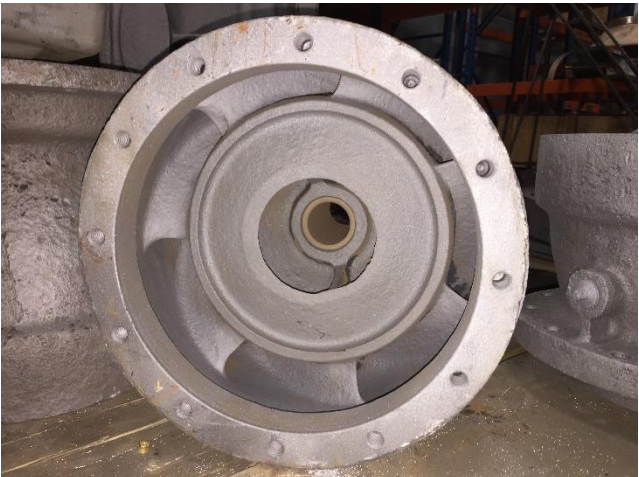
6. Diffuser fit bore and corroded vanes.
