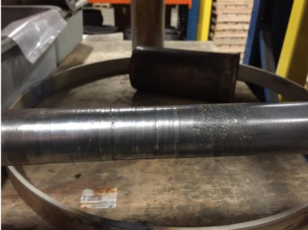
2. Worn and undersize journal turns on upper shaft.
