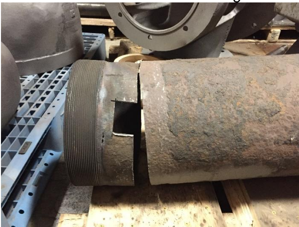
8. Cut column for disassembly.
