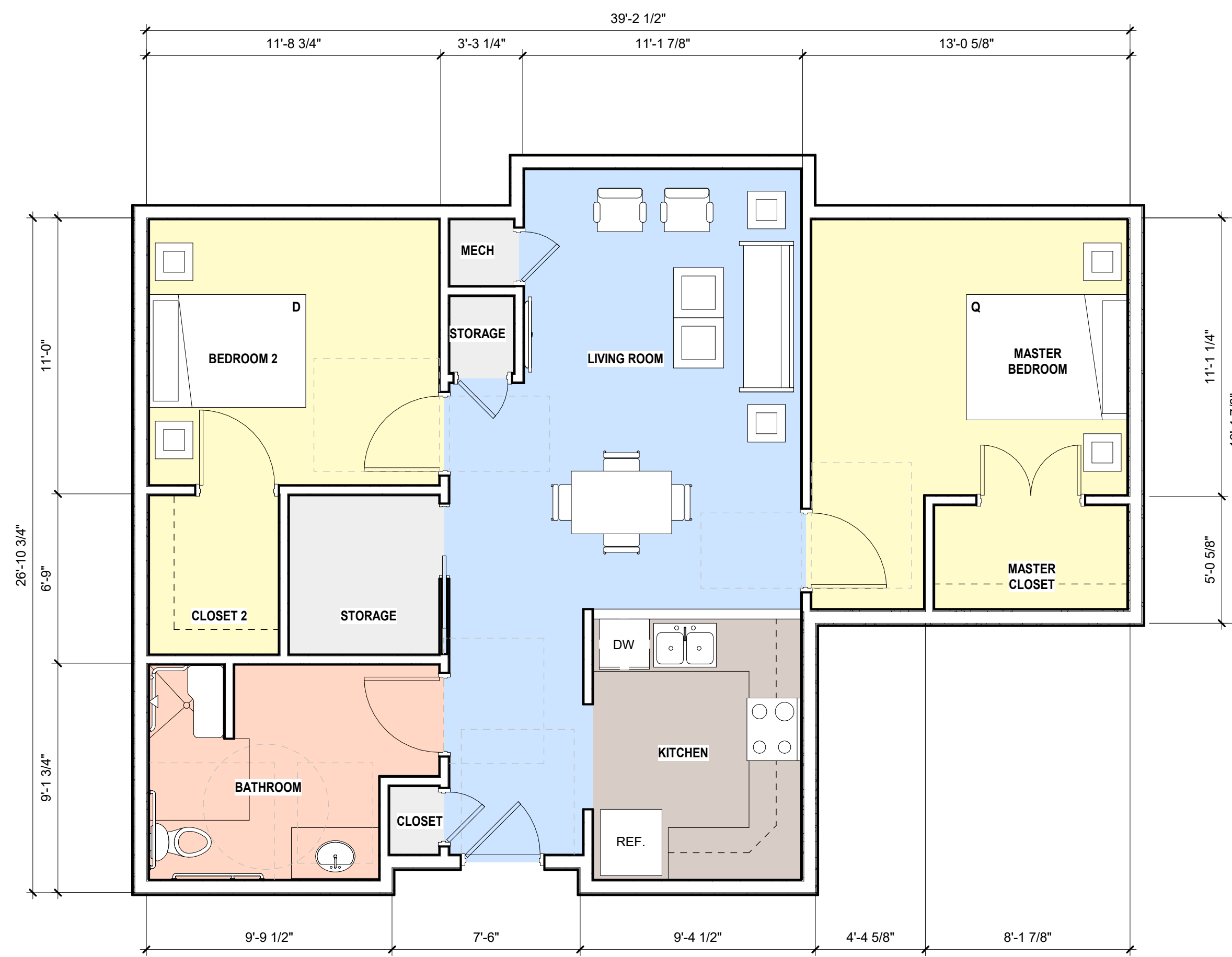
2 UNIT PLAN - 2-BED (900SF) SCALE: 1/4" = 1'-0"
