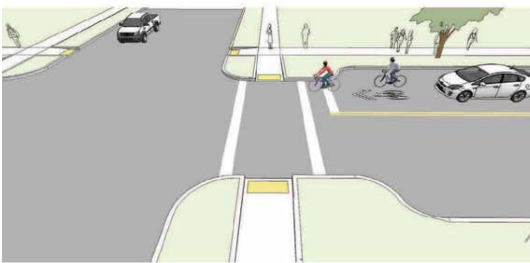
Figure 5.4: Intersection Concepts: Neckdowns
