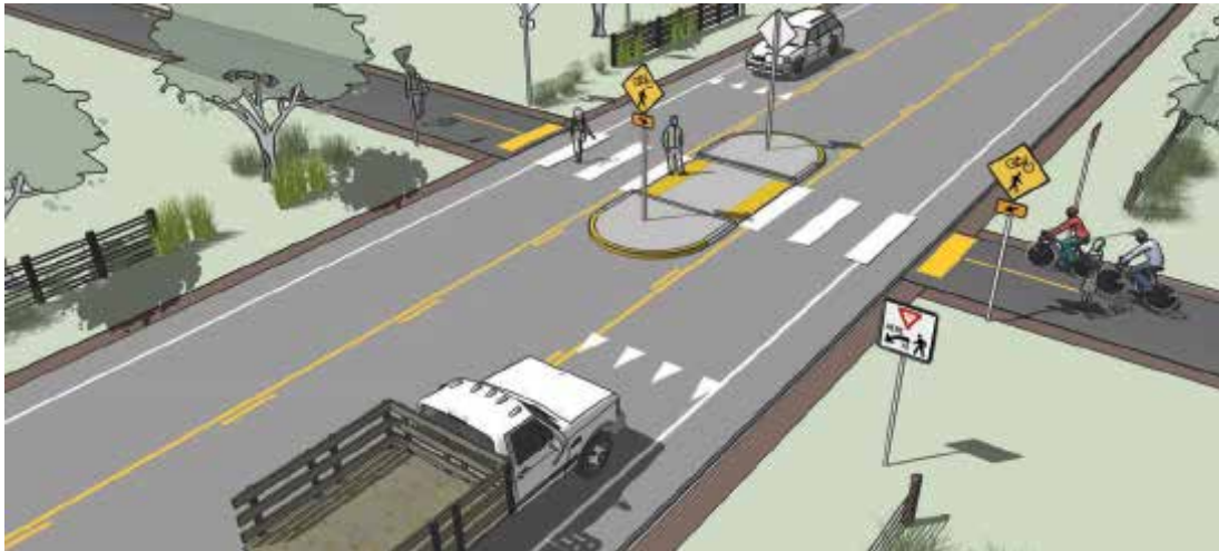
Figure 5.7: Intersection Concepts: Pedestrian Refuge Median
