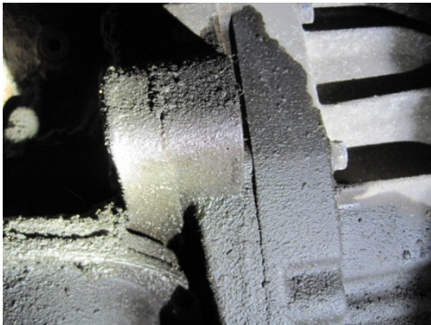
Engine oil leak
