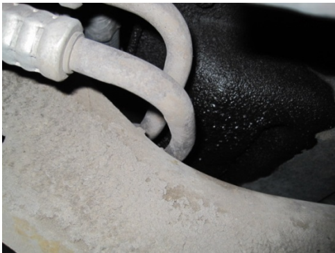
Rear engine oil leak
