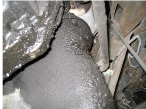
Front engine oil leak
