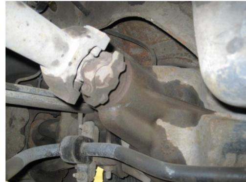
Pinion seal on rear axel
