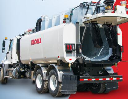
Popular options include a sludge pump to remove material and a decant line to the front bumper.
