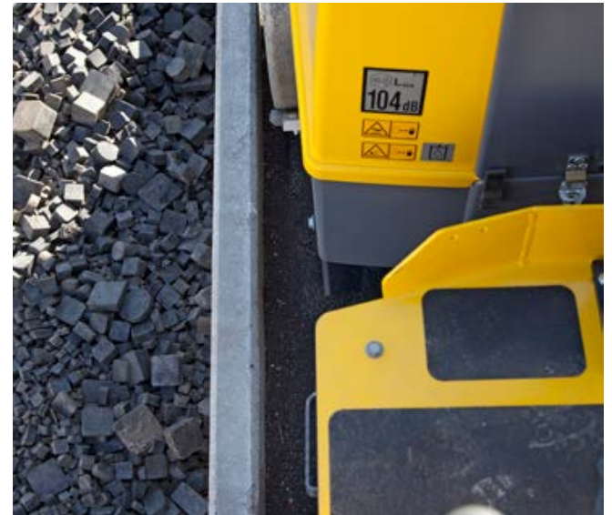
High clearance of the edge of the drums facilitates compaction close to high curbstones. Excellent view over the drum edges for better control and compaction results.
