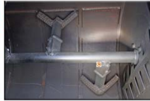
Staggered, angled agitation blades for thorough material blend and to sustain aggregate suspension
